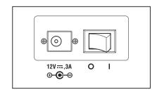
2. Connect the AC adapter plug to the AC adapter input terminal of the body.
